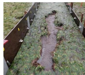
Figure 2: Erosion damage due to wave overtopping
