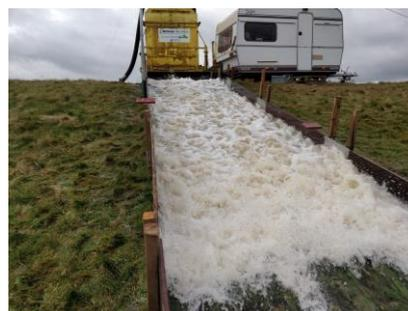
Figure 1: Wave overtopping simulated with the wave run-up simulator
