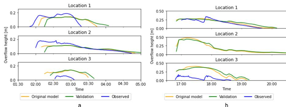
Figure 1 Temporal validation for rainfall events 1 (a) and 2 (b). Overflow height is the water level downstream of a sewage overflow location. Simulation results are close to the original model. Simulations at Location 3 do not match observed values. For Location 2 in Figure b, no observational data was available.
