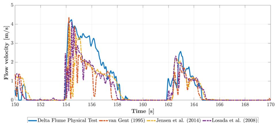
Figure 1: Observed and modelled flow velocity using resistance coefficients of Van Gent (1995), Jensen et al. (2014) and Losada et al. (2008).
