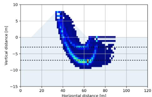
Figure 2: Variation in the location of the critical slip plane.
