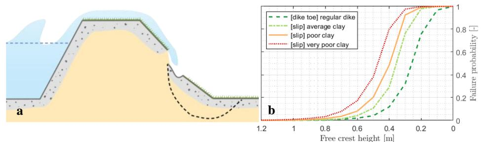
Figure 1: Failure by macro-stability with wave overtopping: (a.) erosion of the grass cover on the slipped dike (b.) fragility curve for a slipped dike profile compared to erosion at the dike toe following the Hoffmans model.
