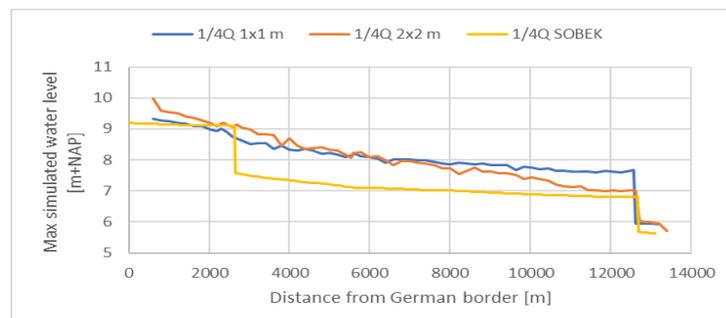
Figure 1: The influence of different grid cell sizes on the simulated water levels in the 1/4Q scenario. The 2x2 m grid (orange line) results in a steeper water level slope compared to SOBEK (yellow line). The water level slope complies with SOBEK in the 1x1 m grid (blue line). However, the water levels are still significantly larger compared to SOBEK.
