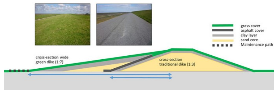
Figure 1: Cross section of a traditional dike and a wide green dike [van Loon-Steensma and Vellinga, 2019]
