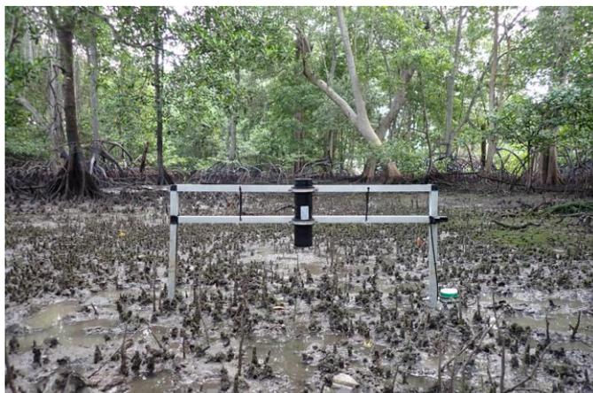
Figure 1: Monitoring station with bed level dynamics and water level instruments in Sungei Buloh Wetland Reserve.
