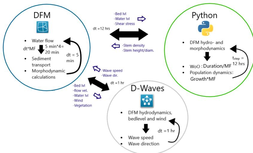
Figure 1: The interaction between the hydrodynamic model (DFM, top left), wave model (D-waves, bottom) and the vegetation model in Python (right) along with the phenomena the separate sections calculate and pass on. MF is a morphological factor which essentially multiplies the bed level change and vegetation development by a factor to enable much faster computation.
