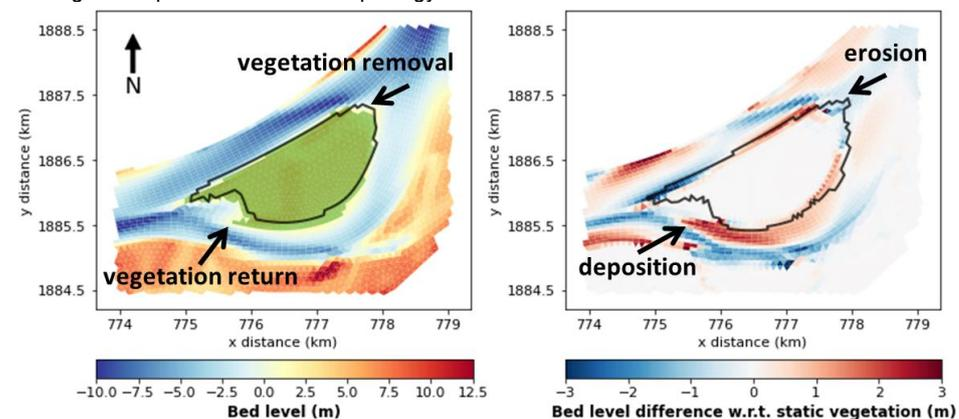
Figure 1: Development of the river bed after one year (left). Bed level difference w.r.t. static vegetation after one year (right). Black lines in left and right panels show the initial location of respectively the vegetation and the mid-channel bar. Green area shows the new location of vegetation after one year.
