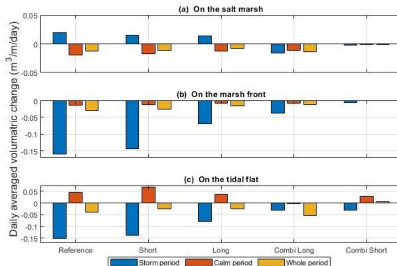
Figure 1: Simulated daily and length averaged volumetric change (a) on the salt marsh, (b) on the salt marsh front and (c) on the tidal flat. The storm period is the combined bed-level change for the storms of 4-5 October 2017 and 27-28 October 2017. The calm period is from 8 to 21 October 2017. The whole period is for the whole simulated month of October 2017.
