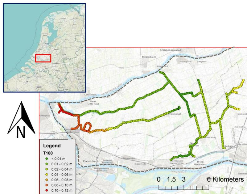
Figure 1: Differences in normative water levels between the dependent and independent situation in the Alblasserwaard area considering all the interdependencies with a return period of 100 years (T100). A positive difference means that the modelled dependent situation has higher normative water levels than the independent case.
