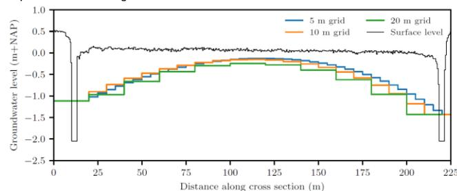
Figure 2: Cross-section of simulated groundwater levels of a farming lot bounded by two ditches in the Waalenburg polder using different sizes for the calculation grid.
