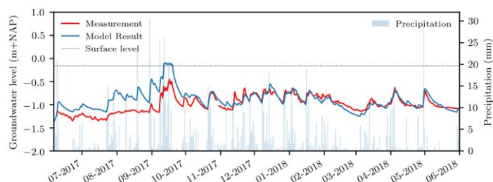
Figure 1: Measured and simulated groundwater levels, the surface level at a measuring well in the Waalenburg polder and daily precipitation at Den Burg.
