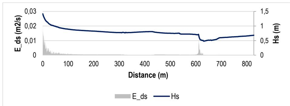
Figure 1 - Wave energy dissipation ( $E_{ds}$ ) and corresponding wave height ( $H_s$ ) along the high wave reducing transect for T=100 years
