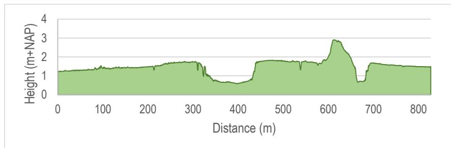
Figure 2 - Elevation profile of the high wave reducing transect
