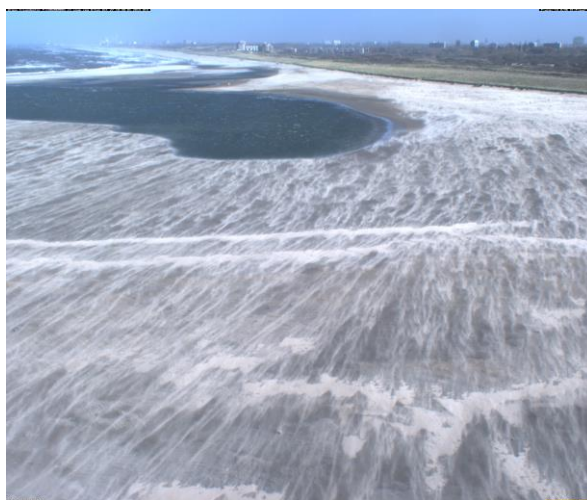
Figure 1: Left) Sand transport in saltation mode over the moist sand surface of the SandMotor nourishment (Argus tower, cam1, 27/10/2013). Right) DPM model snapshots of the erosion process by particle impact.
