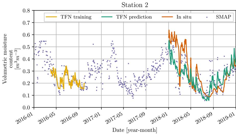
**Figure 4.10:** TFN model results for location 2 when the summer 2016 period is used as training period.
