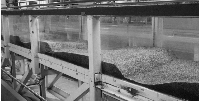
**Figure 1.3:** Dunes formed in a laboratory channel at the University of Auckland (Friedrich *et al.*, 2007). Steady flow was from left to right. It was visually confirmed that there was flow separation present in the dune lees.
