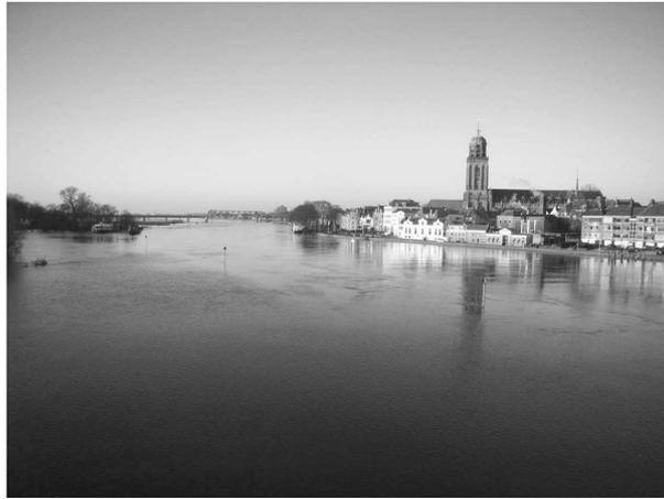
**Figure 1.1:** High discharge event in the river IJssel at Deventer on 16 december 2007 (discharge at Lobith was  $4,500 \text{ m}^3 \text{ s}^{-1}$  and the local water level was  $5.45 \text{ m}+\text{NAP}$ ). The beacons on the picture are located on groynes which are currently below the water surface. At the right bank, the water level is almost at the level of the levees and the floodplain on the left is inundated.
