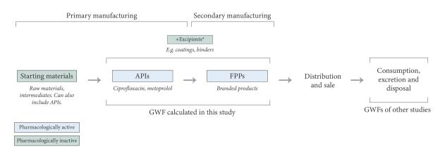
Figure 2: An outline of the pharmaceutical manufacturing supply chain, partly based on Haywood & Glass (2011); ICH (2000); Shah (2004); World Health Organization (2014). \*Although excipients are generally classified as inactive ingredients, they can substantially affect a pharmaceutical's pharmacodynamic and pharmacokinetic properties (Bhattacharyya et al., 2006; Gerber et al., 2018; Haywood & Glass, 2011).
