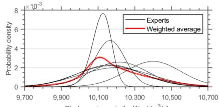
Discharge towards the Waal [m<sup>3</sup>/s] Figure 2: Probability distributions of the discharge distribution towards the Waal.
