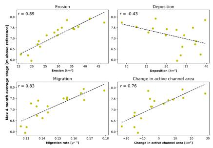
Figure 1: The measured metrics and the relation with the measured average flood season intensity. The average flood season intensity is defined at the maximum 4-month average water level.
