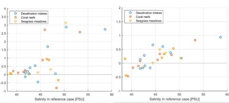
Figure 1: Scatterplot of impact of desalination capacity increase by ten times reference capacity.
