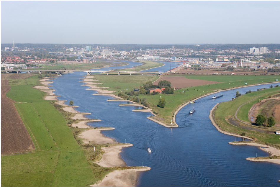
Figure 1.1: IJsselkop bifurcation: one of the two major bifurcations of the Rhine river in the Netherlands (Source: Rijkswaterstaat, 2009). The flow is from the foreground to the background.
