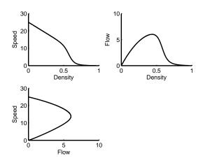
Figure 3: Fundament Diagram obtained with the M/M/1 threshold queue.
