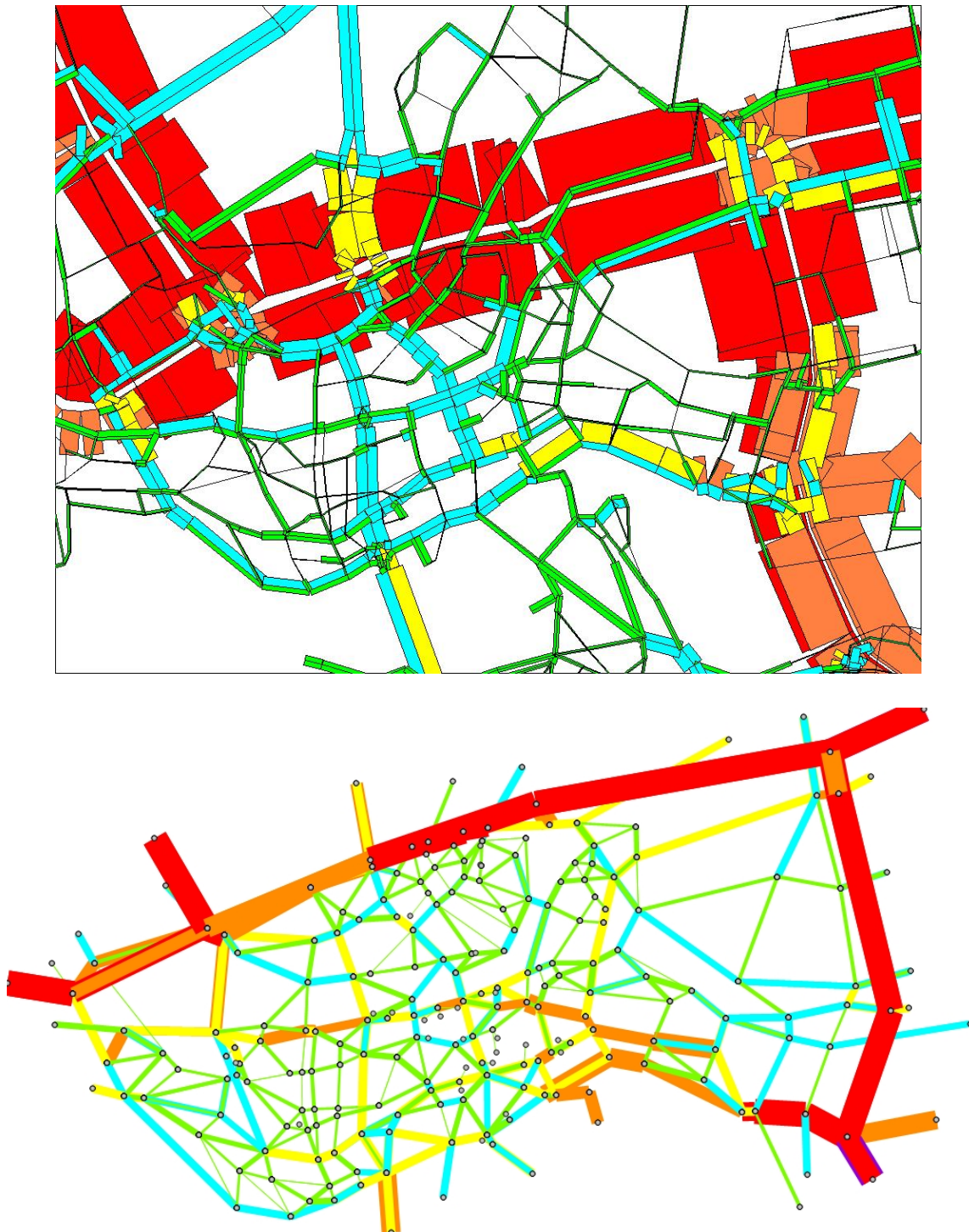
Figure G.6: Comparison of link flows period 15 (top: RBV, bottom: guidance model)
