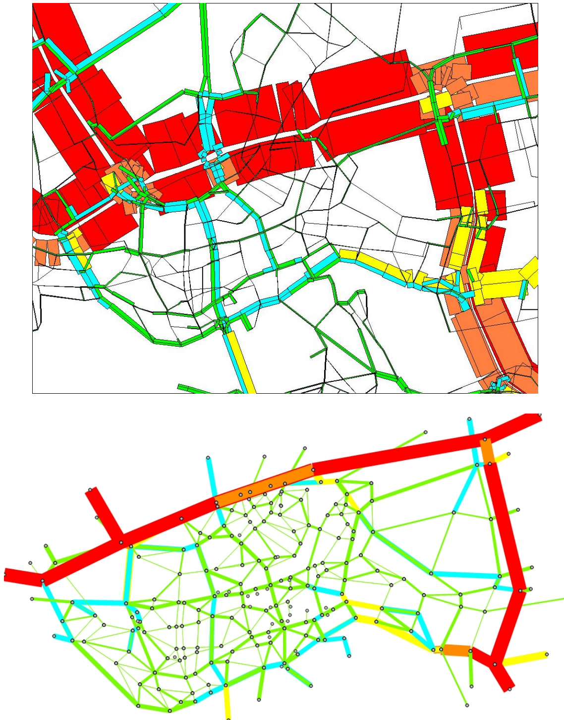
Figure H.2: Comparison of calibrated link flows period 1 (top: RBV, bottom: guidance model)
