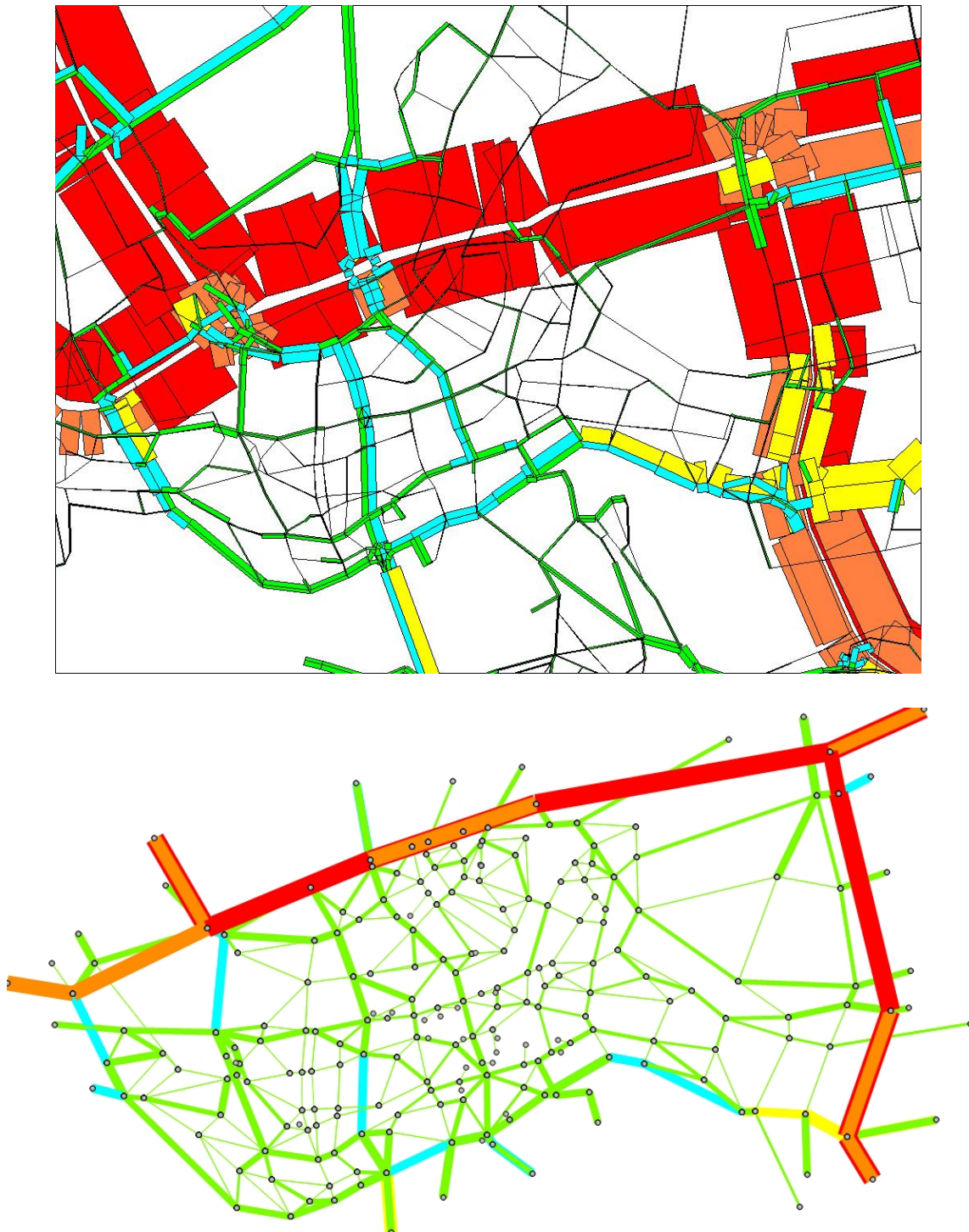
Figure G.2: Comparison of link flows period 1 (top: RBV, bottom: guidance model)
