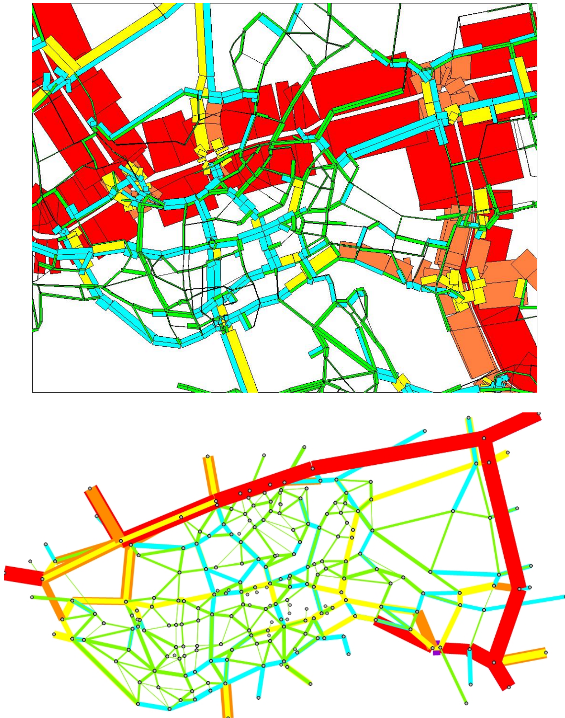
Figure G.4: Comparison of link flows period 8 (top: RBV, bottom: guidance model)
