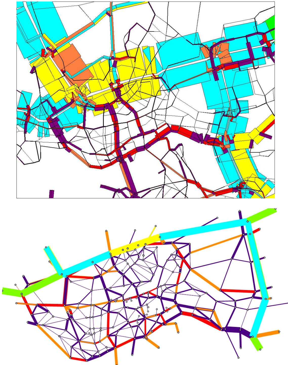
Figure H.3: Comparison of calibrated link speeds period 1 (top: RBV, bottom: guidance model)
