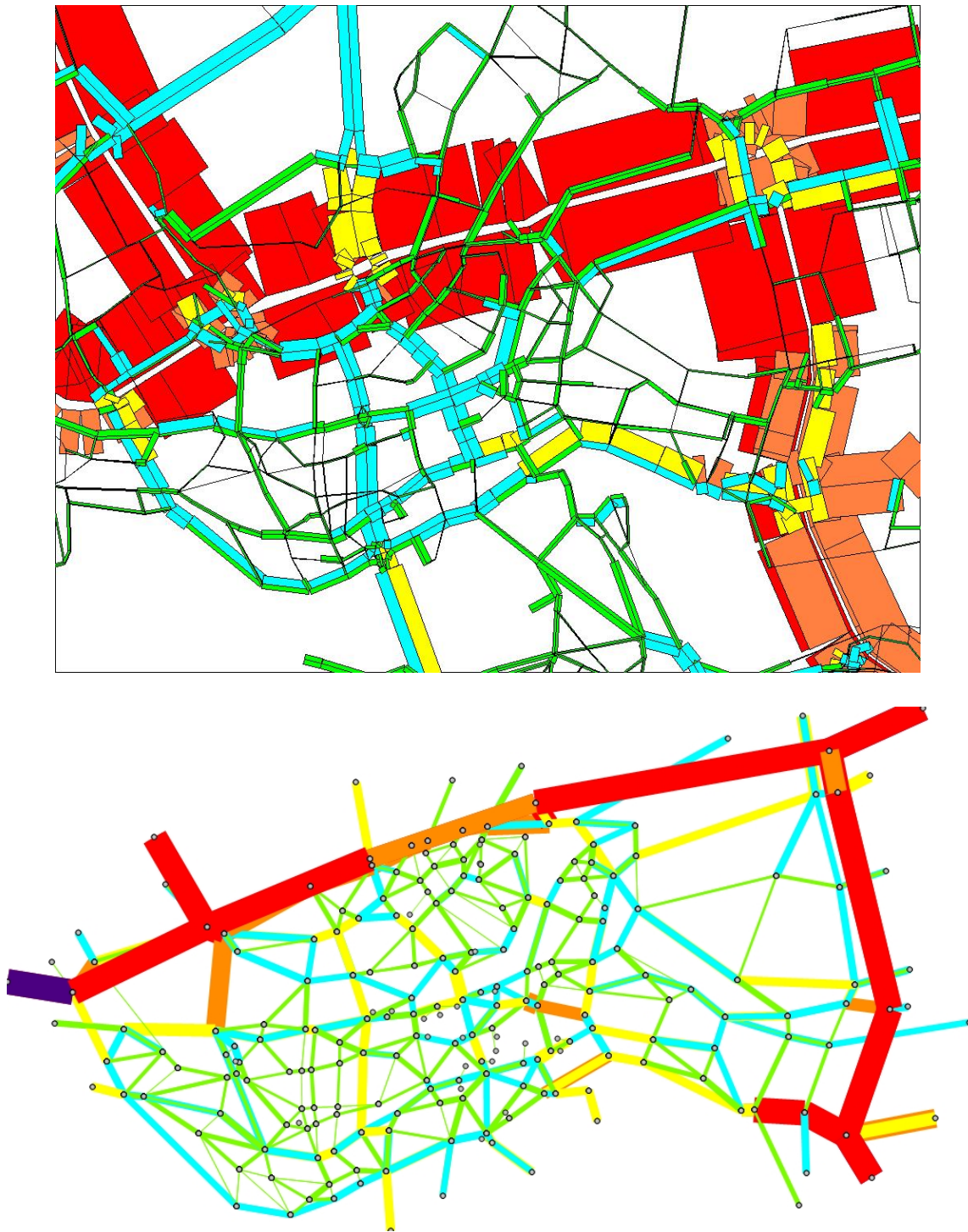
Figure H.6: Comparison of calibrated link flows period 15 (top: RBV, bottom: guidance model)
