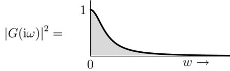
Since the magnitude of  $G$  is monotonically decreasing, the optimal hold-and-sampler combination will cut off the first Nyquist band:
