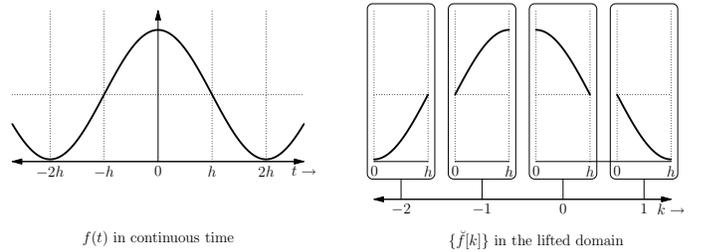
Figure 5: Lifting the analog signal  $f(t) = 1 + \cos(\frac{\pi}{2h}t)$
