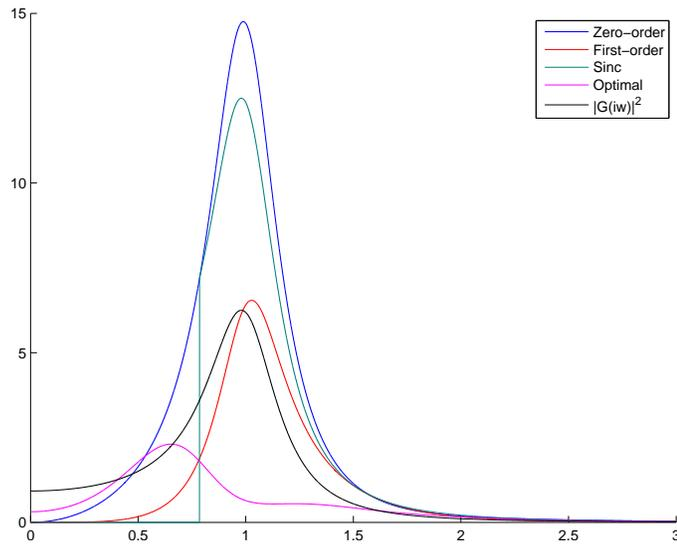
Figure 15: Plots of the FPR of  $(\mathcal{I} - \mathcal{HS})\mathcal{G}$  for  $G(s) = \frac{1}{(s+0.2)^2+1}$ , the ideal sampler and different holds. In blue the zero-order hold, in red the first-order hold, in green the sinc hold, in pink the optimal hold and in black the response of the system itself  $|G(i\omega)|^2$
