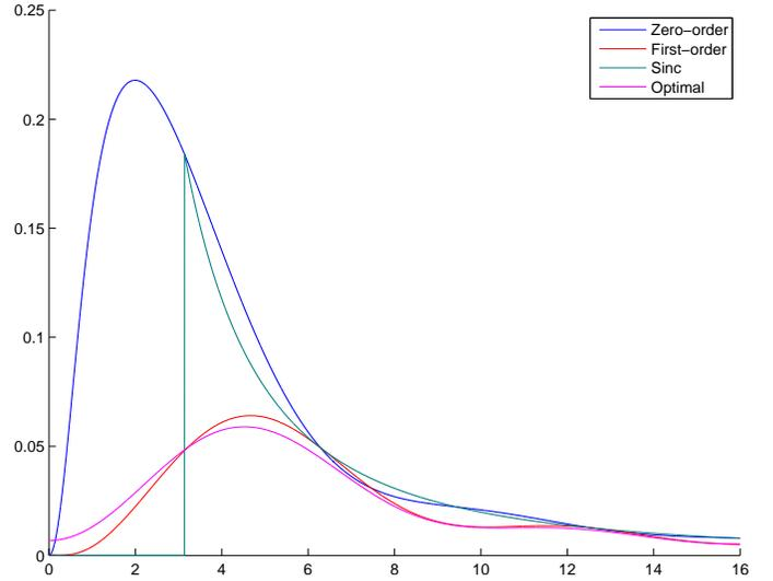
Figure 14: Plots of the FPR of  $(\mathcal{I} - \mathcal{H}\mathcal{S})\mathcal{G}$  for  $G(s) = \frac{1}{s+1}$ , the ideal sampler and different holds. In blue the zero-order hold, in red the first-order hold, in green the sinc hold and in pink the optimal hold
