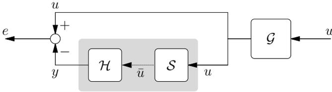
Figure 1: A system with sampler  $\mathcal{S}$ , hold  $\mathcal{H}$ , generator  $\mathcal{G}$ , generator signal  $w$ , input signal  $u$ , sampled input signal  $\bar{u}$ , output signal  $y$  and error signal  $e$
