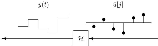
Figure 3: Example of a hold that holds the output constant over one sampling period (zero-order hold)
