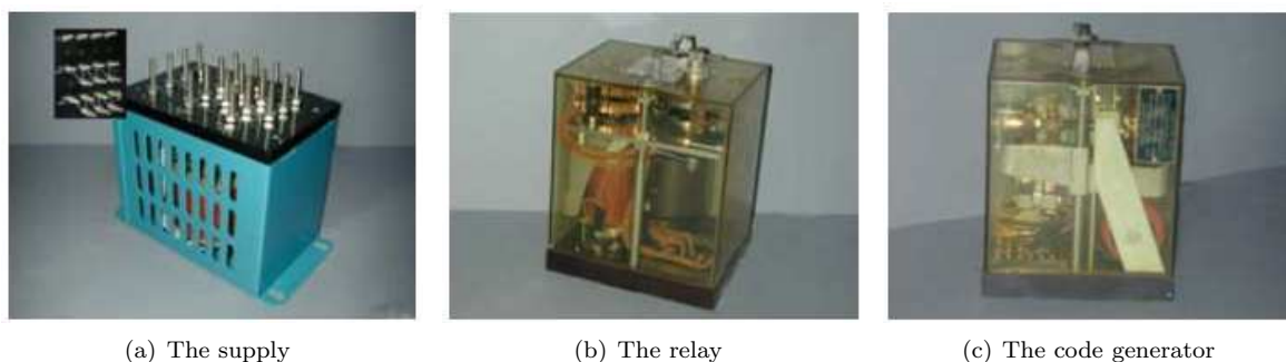
Figure 3.7: Some parts of the measuring arrangement (real size: about 35 cm high)
