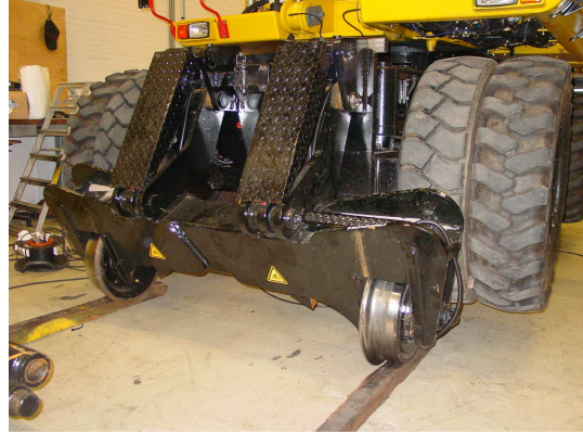
Figure 3.5: The axle of the KROL is 'wrapped around' the wheels
