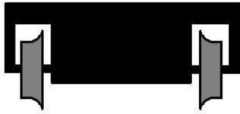
Figure 3.5: The axle of the KROL is 'wrapped around' the wheels
