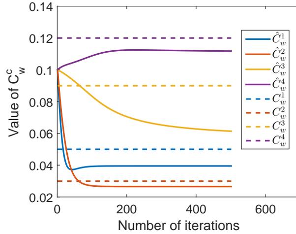
Figure 4.12: Convergence of the process noise variance. The true values are  $C_w^c$  plotted as dashed lines and the estimates  $\hat{C}_w^c$  are the solid lines. The common initial value for the estimates is 0.1 and from there the estimates convergence are not close to the true values.
