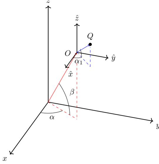
Figure 3.2: The fixed center  $O$  is placed at range  $R_0$  and with azimuth angle  $\alpha$  and elevation angle  $\beta$  in the radar coordinate system. There is a local coordinate frame  $(\hat{x}, \hat{y}, \hat{z})$  with center  $O$  in which the point scatterer  $Q$  is expressed with respect to origin  $O$ .
