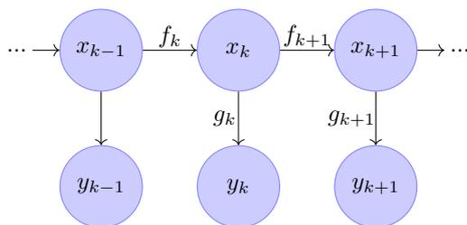
Figure 2.4: The graphical representation of a hidden Markov model, where the arrows represent dependencies between state  $x_k$  and observations  $y_k$ .
