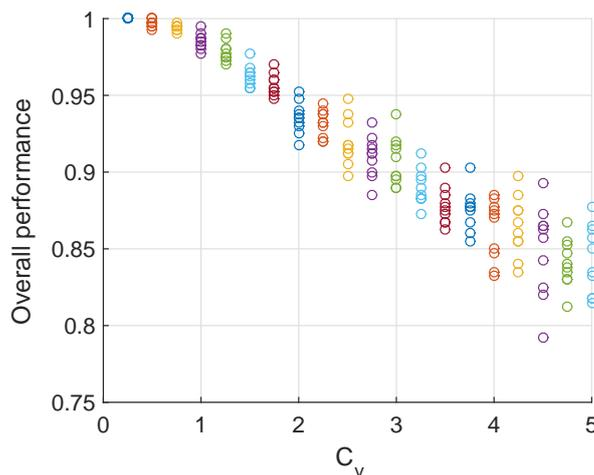
Figure 4.2: This figure shows the degradation of the performance if the measurement noise variance  $C_v$  increases. The observations originate from the 4 classes and the corresponding one point models as described above. For each value of  $C_v$  ten iterations are done to indicate the variance in the performance of the classifier for the same set of parameter values.
