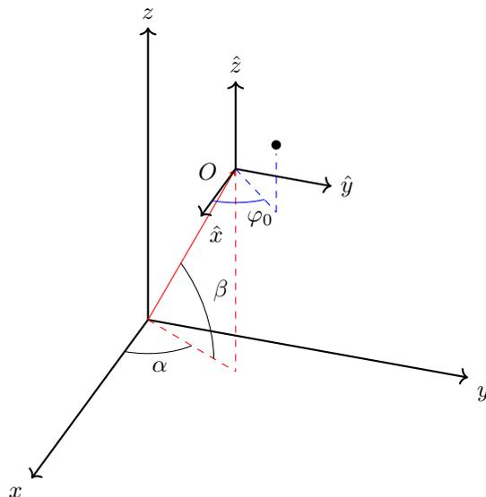
Figure 3.1: The fixed center  $O$  is placed at range  $R_0$  and with azimuth angle  $\alpha$  and elevation angle  $\beta$  in the radar coordinate system. There is a local coordinate frame  $(\hat{x}, \hat{y}, \hat{z})$  with center  $O$  in which the point scatterer  $P$  is expressed with respect to origin  $O$ .
