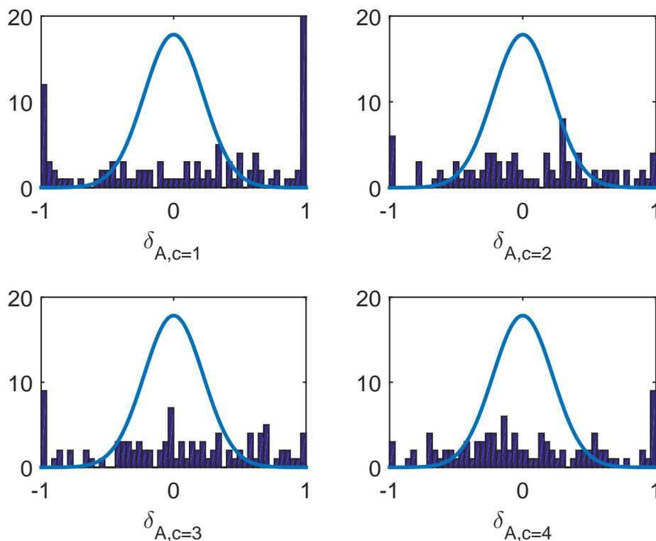
Figure 4.15: Histograms of estimates of the bias  $\delta_A^n$ . One histogram for each class  $c$  with all observations that are classified into class  $c$ . The underlying true density function is also plotted.
