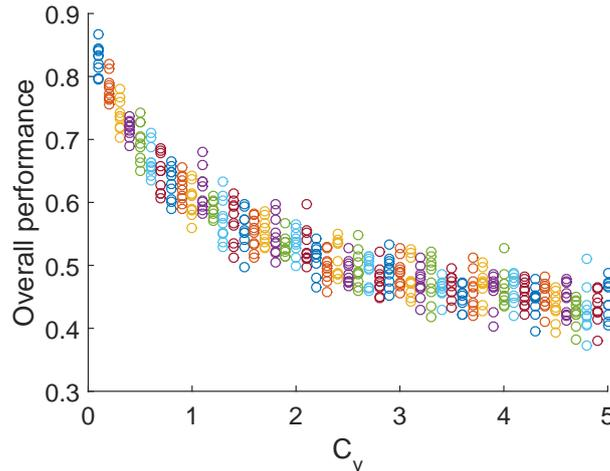
Figure 4.7: This figure shows the degradation of the performance if the measurement noise variance  $C_v$  increases. The observations originate from the four classes and the corresponding rotor and double wing models as described above. For each value of  $C_v$  ten iterations are done to indicate the variance in the performance of the classifier. The ten iterations are plotted in the same color.
