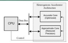
Figure 2. Our design methodology for iterative algorithms enables initial iterations to be processed on an approximate core (while the rest on an accurate core) to achieve an overall energy-efficiency.
