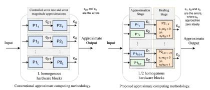
Figure 3. The proposed self-healing methodology [5] does not restrict the approximations based on an error profile but provides the opportunity for error cancellation to achieve an effective quality-efficiency trade-off.
