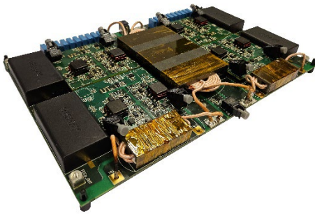
GaN-CLLC Converter in the PE Lab (3 kW)
