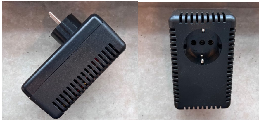
Figure 2. The photo of the Power Quality monitoring device.
