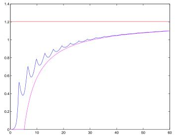
Figure 11: In red the  $L^2$ -norm of  $\mathcal{G}$ ; m(h), in blue the  $L^2$  norm of the error system  $(\mathcal{I} - \mathcal{HS})\mathcal{G}$ ; p(h) and in pink the difference between the  $L^2$ norm and the scaled  $L^{\infty}$  norm of  $\mathcal{G}$ ; q(h). On the horizontal axis the sampling period h and on the vertical axis the size of the norm. Here it is clear that q(h) is indeed a lower bound for  $||(\mathcal{I} - \mathcal{HS})\mathcal{G}||$
