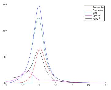
Figure 15: Plots of the FPR of  $(\mathcal{I} - \mathcal{HS})\mathcal{G}$  for  $G(s) = \frac{1}{(s+0.2)+1}$ , the ideal sampler and different holds. In blue the zero-order hold, in red the first-order hold, in green the sinc hold, in pink the optimal hold and in black the response of the system itself  $|G(i\omega)|^2$
