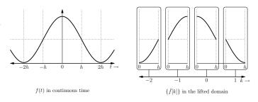
Figure 5: Lifting the analog signal  $f(t) = 1 + \cos(\frac{\pi}{2h}t)$
