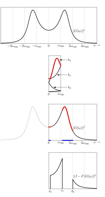
Figure 9: Unfolding the response of  $|G(i\omega)|^2$  after determining the maxima (red). In blue the frequencies that will be filtered in order to achieve a minimal  $L^2$  norm of the error system. There is one unfiltered band  $[\delta_1, \epsilon_1]$  and the tail  $[\delta_n, \infty)$ , so in this case *n* equals 1
