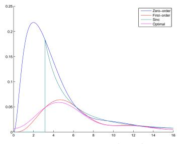
Figure 14: Plots of the FPR of  $(\mathcal{I} - \mathcal{HS})\mathcal{G}$  for  $G(s) = \frac{1}{s+1}$ , the ideal sampler and different holds. In blue the zero-order hold, in red the first-order hold, in green the sinc hold and in pink the optimal hold
