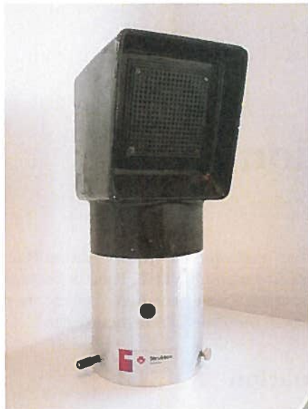
Figure 1.1: Warning bell of railroad crossing with camera (the black circle above the logo)
