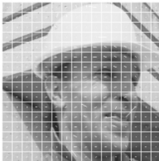
Figure 1.1: Reference frame with macroblocks and motion vectors (from [15])
