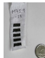
Fig. 4: Magnetic polymer patterned on textile [23].
