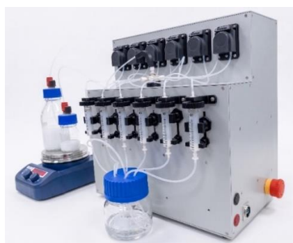
Figure 1: ColumnPack instrument: automated packing of DMC columns
