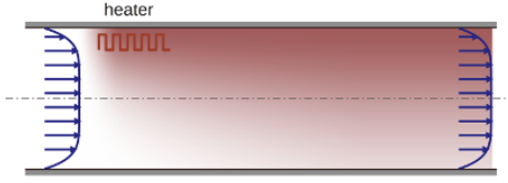
Figure 1. Schematic of a locally heated channel with a non-Newtonian fluid flow.
