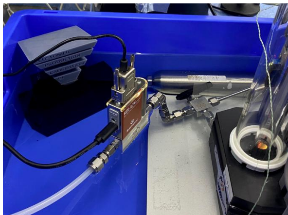
Figure 2: Body of FLEXI-FLOW Compact is also submersed in water to eliminate environmental effects.
