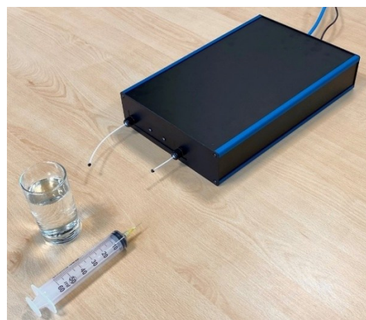
Figure 1: The compact NMR system shown together with a glass of water and a 60 ml syringe as scale reference.
