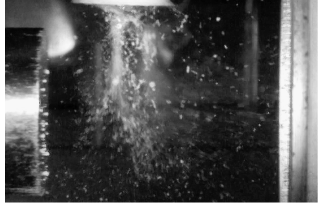
Figure 4: Standing-wave atomization of silicone oil with viscosity of 1,000 \text{ cSt} ( 960 \text{ mPas} ) at a mass flow of 2.5 \text{ ml/s}
