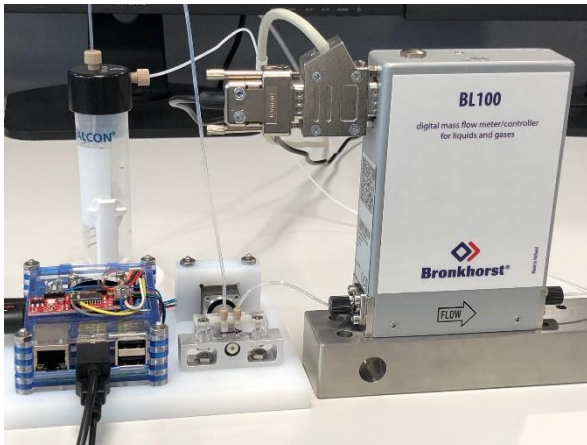
Figure 2: Measurement set-up consisting of the MSM micropump (left) and Bronkhorst's Micro Coriolis Mass Flow Meter BL100 (right).
