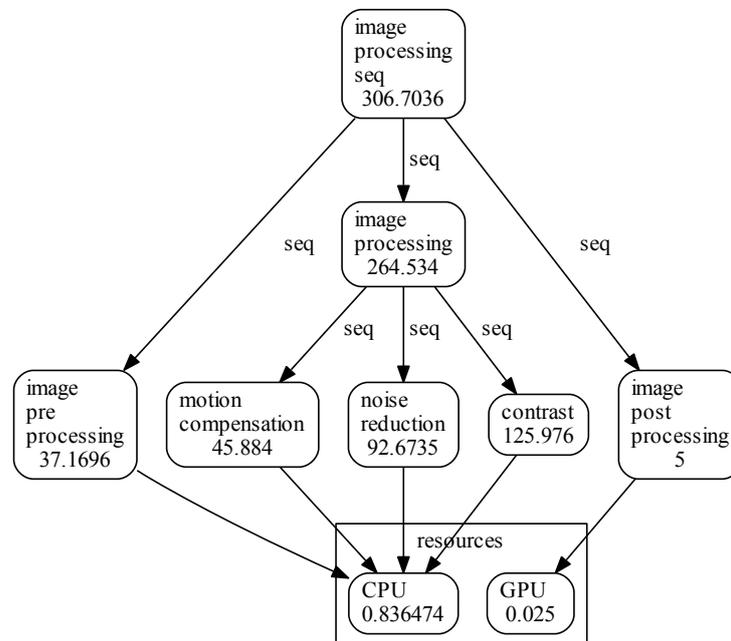
■ **Figure 5** The latency breakdown chart and utilization (offset=0), based on MODES simulation results, which is automatically generated from the iDSL code.
