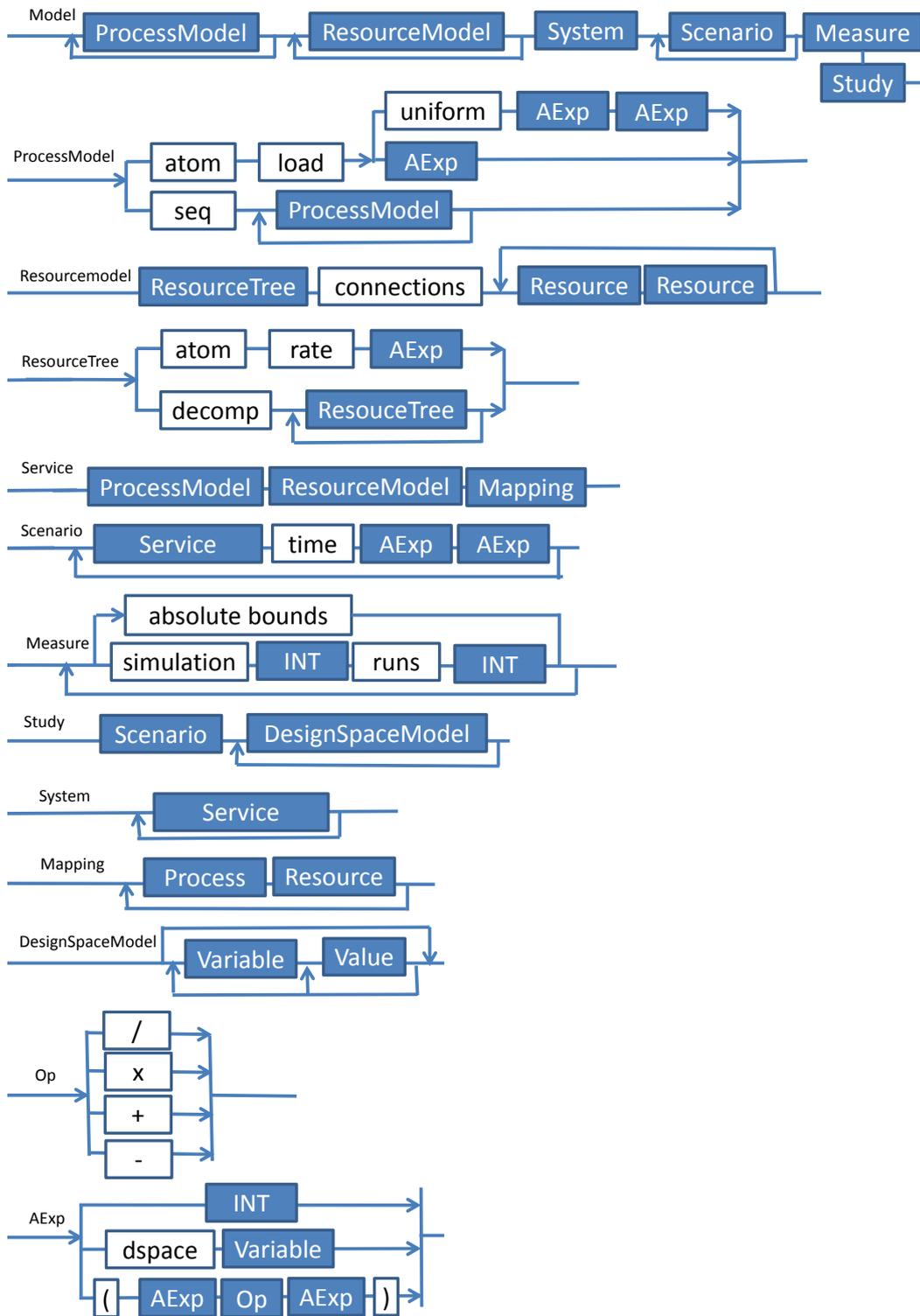
■ **Figure 9** The grammar of iDSL's language as used in this paper. The grammar has the *Model* concept as its top-level node. It decomposes into one or more *ProcessModels*, *ResourceModels*, a *System* (a set of *Services*), *Scenarios*, and a *Measure* and a *Study*.
