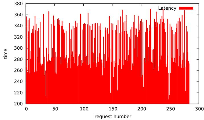
■ **Figure 6** The MODES latency times bar graph (offset=0) for 280 service requests, which is automatically generated from the iDSL code.
