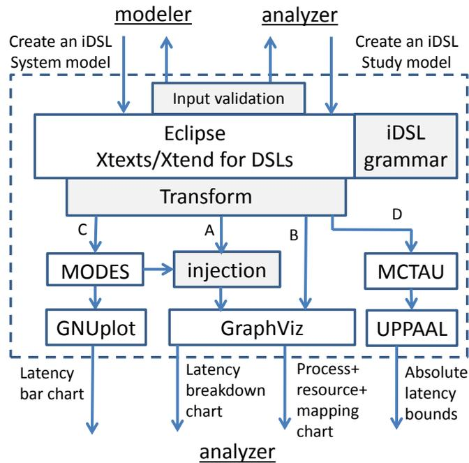
■ **Figure 4** The iDSL tool chain overview. A modeller and analyser create an iDSL model based on the iDSL grammar. The iDSL tool transforms this model into MoDeST and GraphViz models, leading to performance measures to be evaluated by the analyser.
