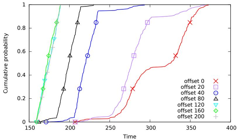
■ **Figure 7** The cumulative distribution functions of latencies for seven design instances is automatically generated from the iDSL code.
