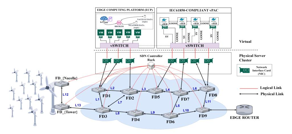
An out-of-band control SDN-Enabled IIoT-Edge network schematic illustrating the fiber-optic-based connectivity between a fleet of wind turbine generator nacelle and tower switches connected to the offshore hub's data center switches FD{1,...,9} leading to the server cluster's physical network interfaces and virtualized networks within the ECP and vPAC nodes.
