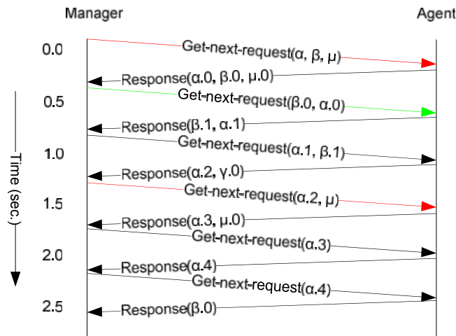
Figure 2.8: TSD showing the changing of positions of OIDs and the irregular insertion of an extra OID
