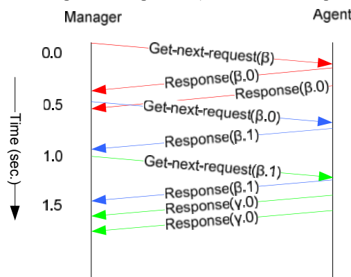
Figure 2.5: Standard retransmissions of responses
