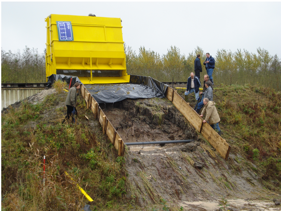
Fig. 4.2: Luisterbuis exposed, after a succesfull test
