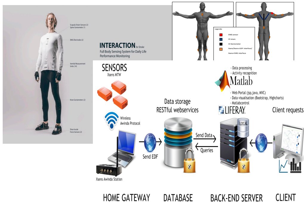
Figure 3. The different components of the Interaction monitoring system ( https://www.xsens.com/news/interaction-project/ )
