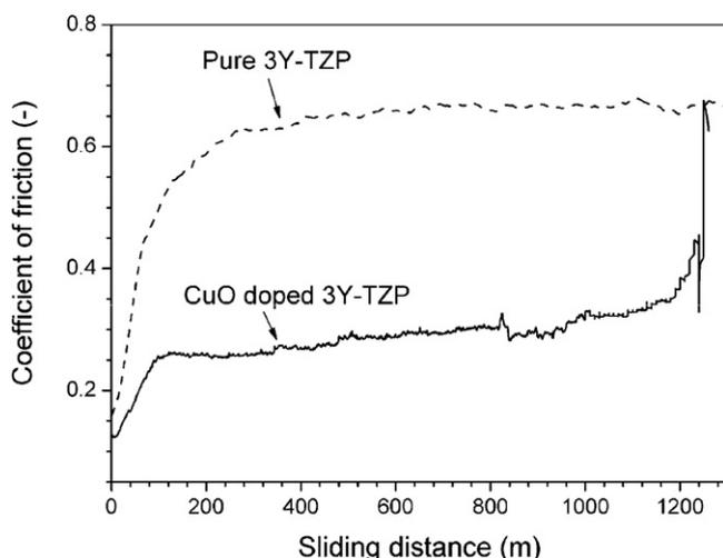
Fig. 1. Coefficient of friction of undoped and 8 mol% CuO doped 3Y-TZP ceramics, when sliding against an alumina ball, as a function of sliding distance.
