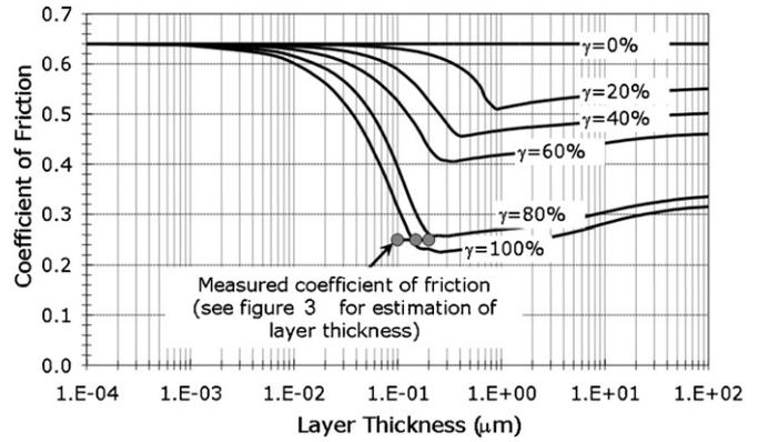
Fig. 8. Coefficient of friction of CuO doped 3Y-TZP sliding against alumina calculated according to Pasaribu's friction model as a function of thickness and coverage of the soft layer in wear track [9].
