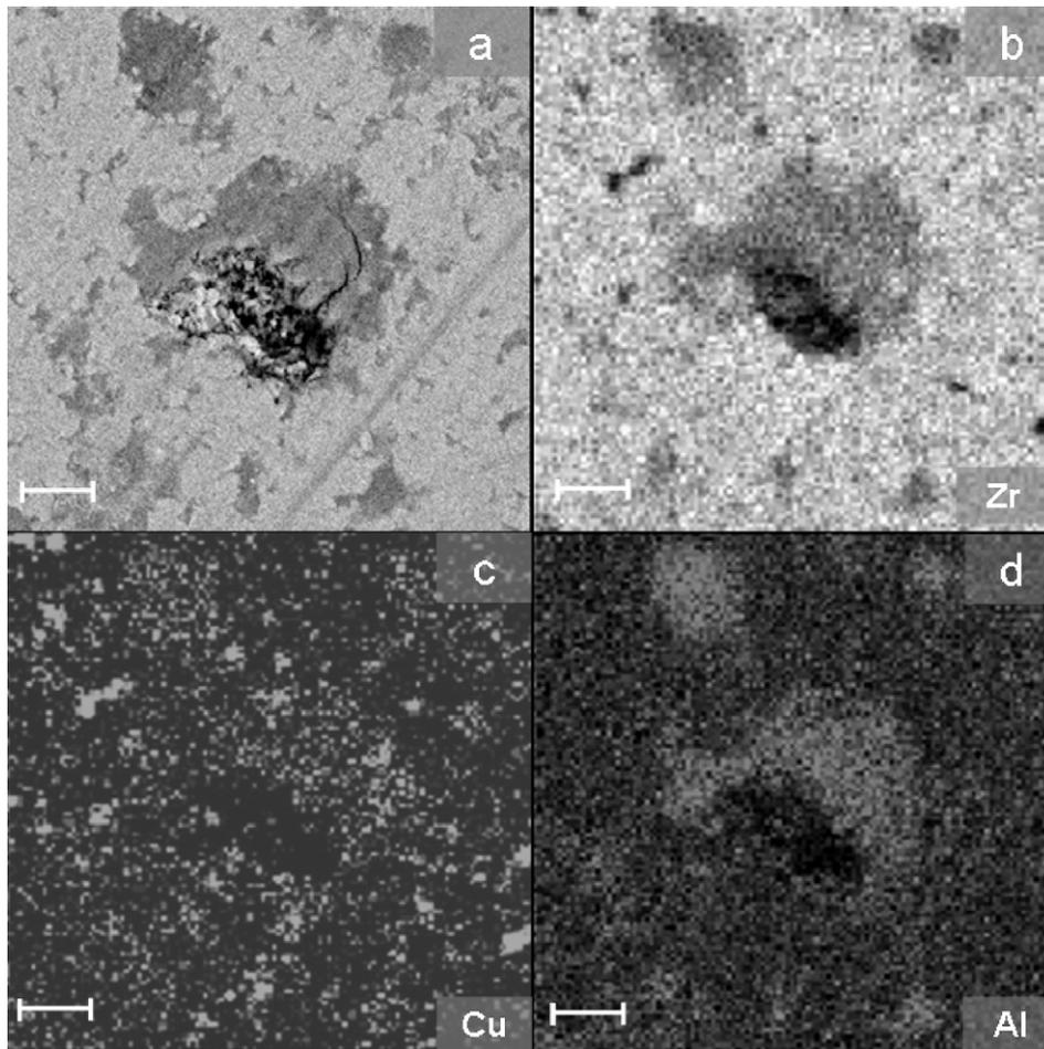
**Fig. 5.** Elemental distribution as determined by EDX mapping of the wear track as shown in Figs. 2 and 4. The bar represents 5  $\mu\text{m}$ . (a) Back-scattered image; (b) Zr distribution; (c) Cu distribution; (d) Al distribution.
