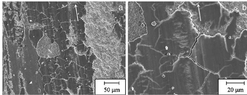
**Fig. 9.** SEM images of the wear track after tribological test for a sliding distance 1.5 km. White arrows in the images denote the sliding direction. (a) Lower magnification; (b) higher magnification.
