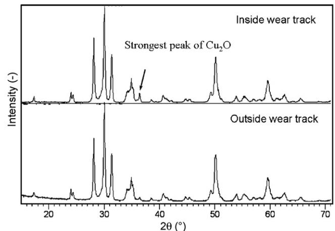
**Fig. 6.** XRD pattern measured in and out the wear track on the 8 mol% CuO doped 3Y-TZP ceramic after tribological test.
