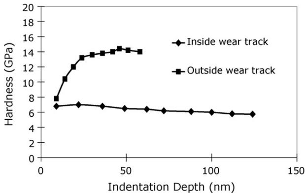
Fig. 7. Hardness as a function of indentation depth of CuO doped 3Y-TZP ceramic after tribological test.
