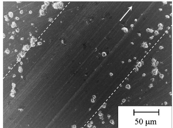
Fig. 2. SEM taken from a 3Y-TZP doped with 8 mol% CuO, after tribological test for around 0.2 km. The weak track is denoted within the two white dot lines and sliding direction is denoted by the white arrow.
