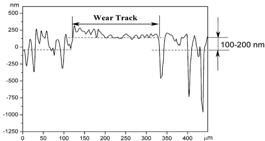
Fig. 3. Surface profile across the wear track after 0.2 km sliding (8 mol% CuO doped 3Y-TZP).
