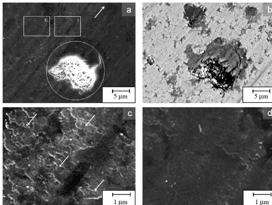
Fig. 4. Higher magnification SEM images of the same wear track as shown in Fig. 2. (a) Secondary electron image, white arrow denotes the sliding direction; (b) back-scattered electron image; (c) enlarged image of area I in a), white arrows denotes micro-fracture pattern; (d) enlarged image of area II in a).
