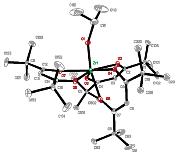
Figure 4. Molecular structure of \text{Zr}(\text{O}^i\text{Pr})(\text{thd})_3 ( 3 ). Selected bond lengths of 3 : \text{Zr}(1)-\text{O}(1) = 1.847(8)\text{ \AA} , \text{Zr}(1)-\text{O}(5) = 2.017(10)\text{ \AA} , \text{Zr}(1)-\text{O}(7) = 2.091(8)\text{ \AA} , \text{Zr}(1)-\text{O}(3) = 2.108(7)\text{ \AA} , \text{Zr}(1)-\text{O}(2) = 2.123(8)\text{ \AA} , \text{Zr}(1)-\text{O}(6) = 2.165(8)\text{ \AA} , \text{Zr}(1)-\text{O}(4) = 2.185(8)\text{ \AA} . The corresponding bond lengths of the hafnium isomorph \text{Hf}(\text{O}^i\text{Pr})(\text{thd})_3 ( 5 ) are as follows: \text{Hf}(1)-\text{O}(1) = 1.810(12)\text{ \AA} , \text{Hf}(1)-\text{O}(5) = 2.050(13)\text{ \AA} , \text{Hf}(1)-\text{O}(3) = 2.116(12)\text{ \AA} , \text{Hf}(1)-\text{O}(7) = 2.123(12)\text{ \AA} , \text{Hf}(1)-\text{O}(6) = 2.154(12)\text{ \AA} , \text{Hf}(1)-\text{O}(2) = 2.165(12)\text{ \AA} , \text{Hf}(1)-\text{O}(4) = 2.161(14)\text{ \AA} .
