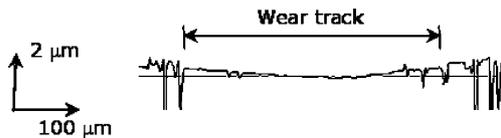
Fig. 3. Typical wear track profile of alumina doped with CuO sliding against alumina at 23 °C and different humidities.
