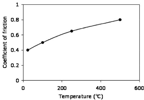
Fig. 5. Coefficient of friction of alumina doped with 5% wt CuO sliding against alumina at elevated temperatures. (Normal load: 5 N and sliding velocity: 0.1 m/s.)
