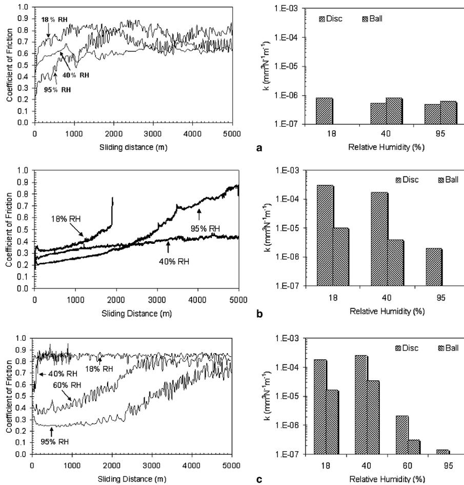
Fig. 4. Coefficient of friction and specific wear rate of pure zirconia (a), zirconia doped with CuO sintered at 1500 °C (b), and zirconia doped with CuO sintered at 1550 °C (c) sliding against alumina at different humidities. (Normal load: 5 N, sliding velocity: 0.1 m/s, temperature: 23 °C.)
