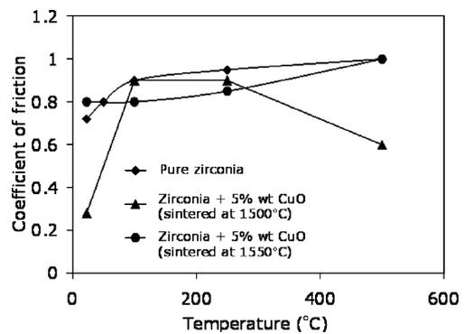
Fig. 6. Steady state coefficient of friction of pure zirconia and zirconia doped with CuO sliding against alumina at elevated temperatures. (Normal load: 5 N and sliding velocity: 0.1 m/s.)
