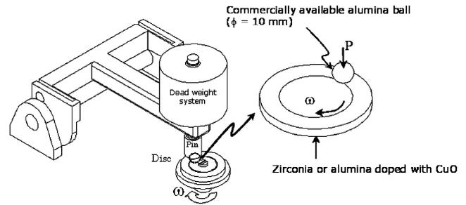
Fig. 1. Schematic representation of the pin-on-disc friction tester.
