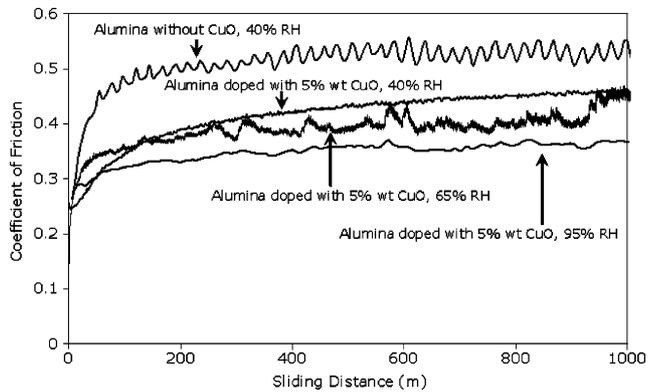
Fig. 2. Coefficient of friction of pure alumina and alumina doped with CuO sliding against alumina at different humidities. (Normal load: 5 N, sliding velocity: 0.1 m/s, temperature: 23 °C.)
