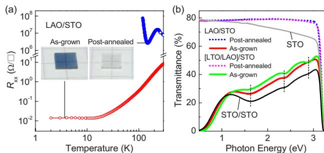
FIG. 1. (Color online) (a) Sheet resistance of LAO (125 unit cells) films on STO substrates. Inset: photographs of as-grown and postannealed LAO/STO samples on  $5 \times 5$  mm<sup>2</sup> mesh paper. (b) Room temperature  $T(\omega)$  of LAO films on STO, [LTO/LAO] superlattices on STO, a STO film on STO, and a bare STO substrate.
