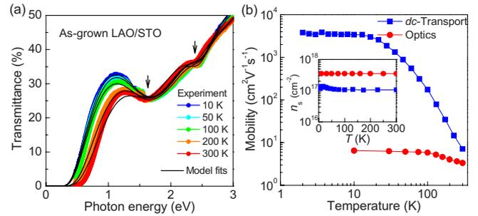
FIG. 3. (Color online) (a) Temperature-dependent  $T(\omega)$  of LAO/STO and their model-fit curves at each temperature. The arrows point the weak absorption bands showing a blue-shift. (b) The mobility as a function of temperature extracted from dc-resistivity and Hall measurements as well as optical transmission spectroscopy. Inset shows  $n_s$  as a function of temperature.
