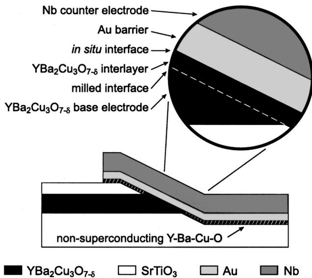
FIG. 1. Schematic cross section of the  $\text{YBa}_2\text{Cu}_3\text{O}_{7-\delta}/\text{Au}/\text{Nb}$  ramp-type junction including the interlayer.
