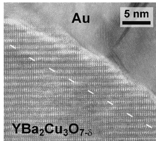
FIG. 2. Bright-field transmission electron microscopy image of the  $\text{YBa}_2\text{Cu}_3\text{O}_{7-\delta}/\text{Au}$  interface at the ramp-edge area, including an interlayer of 6 nm deposited  $\text{YBa}_2\text{Cu}_3\text{O}_{7-\delta}$ . Crystalline  $\text{YBa}_2\text{Cu}_3\text{O}_{7-\delta}$  material is observed up to the Au interface, while no clear interface is observed between the base electrode and the interlayer (dashed line).
