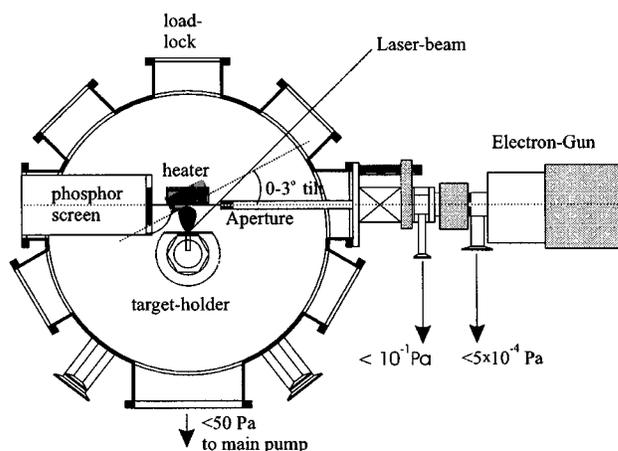
FIG. 1. A schematic view of the deposition chamber, including the electron source assembly.
