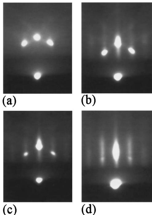
FIG. 2. RHEED patterns of the SrTiO<sub>3</sub> substrate surface in 15 Pa oxygen prior to the growth, (a) at room temperature and (b) at 760 °C and subsequently after deposition of (c) 10 nm of SrTiO<sub>3</sub> and (d) 6 nm of YBCO, both after an *in situ* anneal step at 850 °C.
