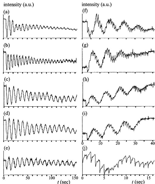
FIG. 3. Intensity oscillations of a diffraction spot during the growth: (a) homoepitaxial growth of SrTiO<sub>3</sub>; (b)–(e) homoepitaxial growth of SrTiO<sub>3</sub> after intermediate *in situ* anneal steps; (f) heteroepitaxial growth of YBCO on SrTiO<sub>3</sub>; (g)–(i) heteroepitaxial growth of YBCO on SrTiO<sub>3</sub> after intermediate *in situ* anneal steps. (j) shows the modulation of the intensity oscillations, due to the laser pulses.
