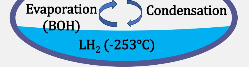
Key idea: small latent heat hydrogen (4.61 kJ/kg [4])  $\rightarrow$  minimal cooling power needed to recondense BOH.
