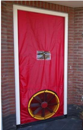
Fig. 1: A fan mounted in the front door of a house for a blower-door-test.
