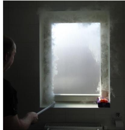
Fig. 2: Smoke to check the infiltration around a bathroom window.
