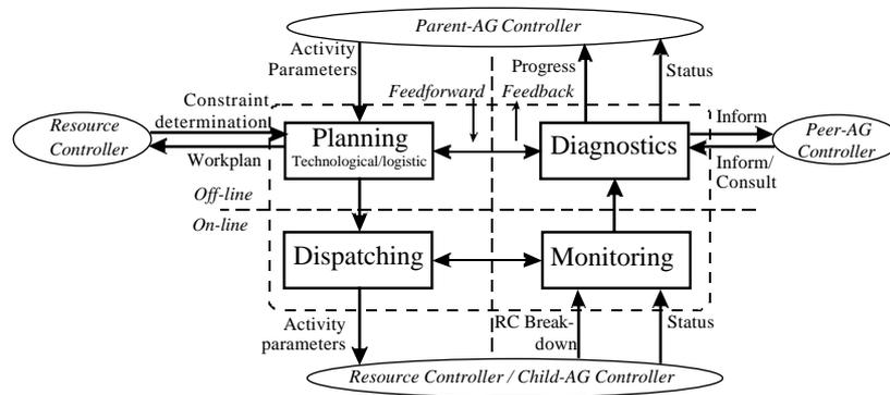
Fig. 4. Functional architecture of the AG Controller [9].
