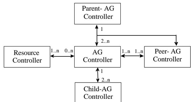
Fig. 3. The framework of the AG and Resource Controllers in the EtoPlan concept.
