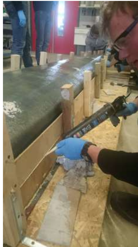
Figure 21: Gluing together the MDF strips
