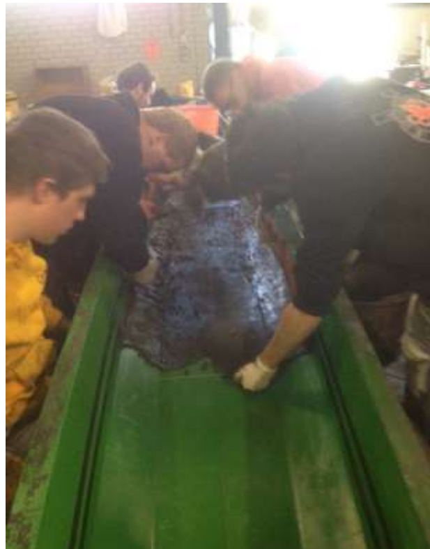
Figure 19: applying the concrete to the canoe
