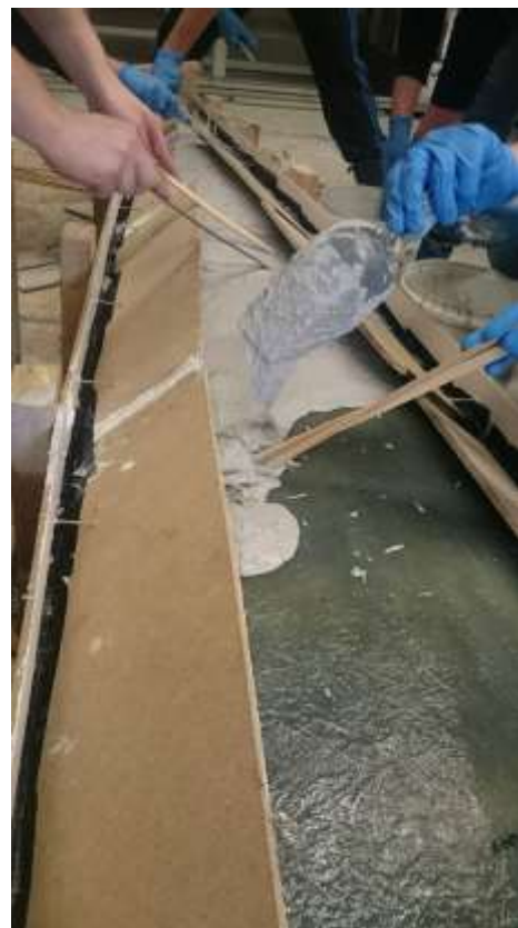
Figure 22: Pouring the floor of the canoe
